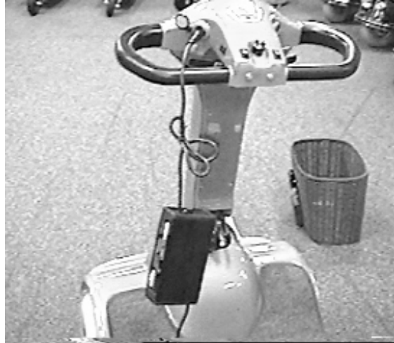
Battery Charger Hook up
