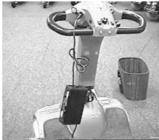
Battery Charger Hook up
