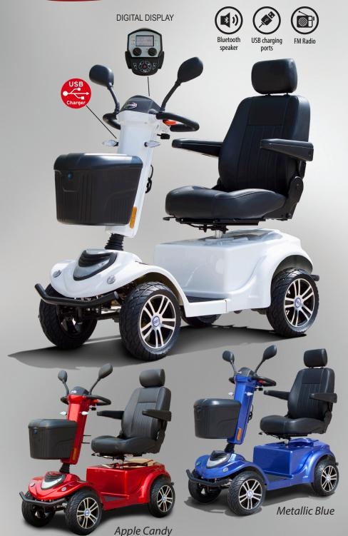
All new Orthoguad RZ1000 establishes a new bench mark for mid-size scooters. Powered by the reliable and powerful high performance 950 watt engine and coupled to 2x 75Ah batteries, it delivers a 15km/h top speed and an impressive range. The RZ1000 offers a high level of comfort even on rugged terrain with its full 4 wheel suspension.
