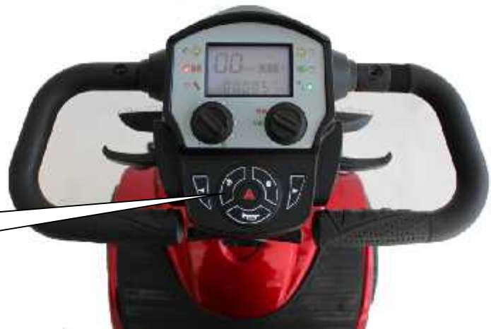
Electric button to release the electromagnetic brake.
